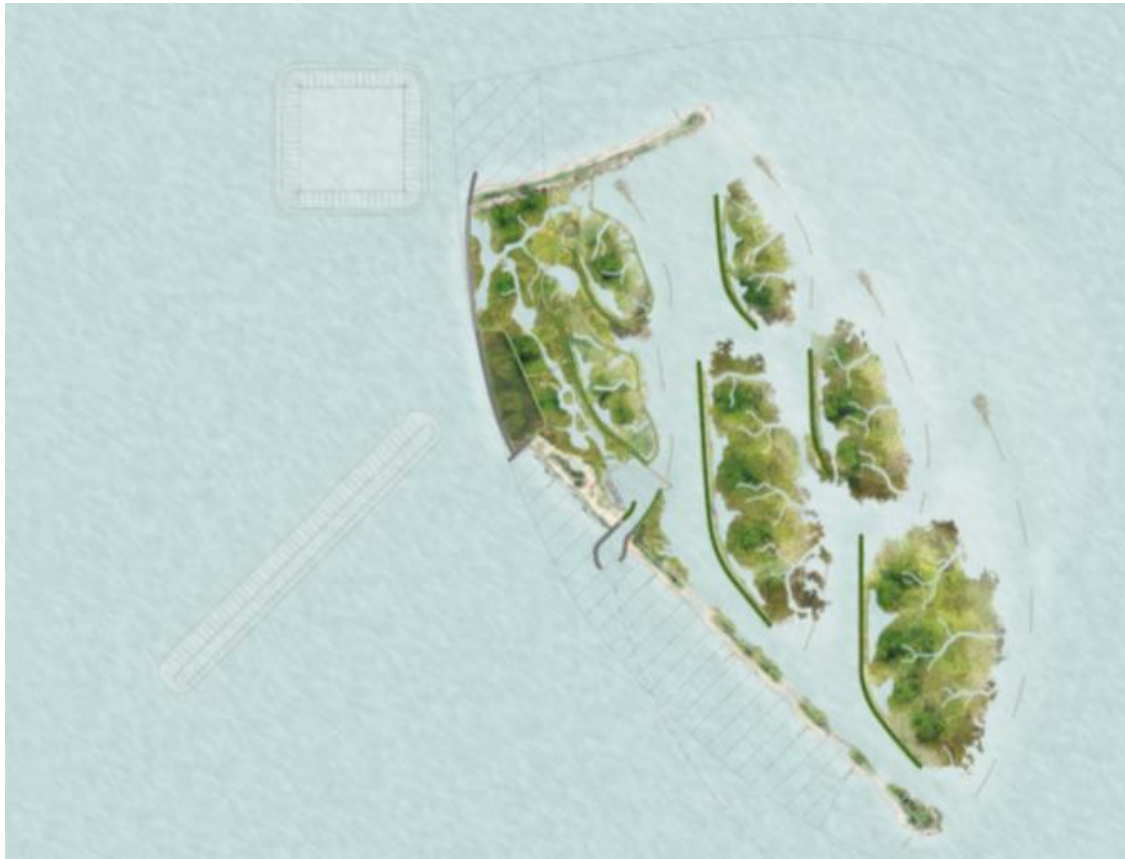
Figure 2 The MW from above, with the sand well in the upper left corner, and the gully to capture fine sediment on the mid left (Boskalis, 2015)
